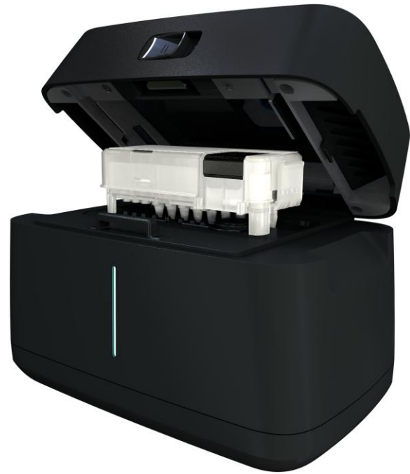
Figure 1. Biomeme M1/Franklin HR-B/V workflow. The system consists of 4 components: an M1 RNA 2.0 sample prep cartridge, 3 Go-Strips panels (A, B, C), the Franklin three9 real-time polymerase chain reaction (PCR) thermocycler, and a smartphone. The M1 sample prep cartridge allows rapid nucleic acid extraction without the need for any equipment. Each Go-Strip consists of 3 connected PCR tubes containing lyophilized master mix, multiplexed primers, and probes for 3 targets. Each handheld unit is equipped with 9 sample wells, enabling simultaneous quantitative detection of up to 27 targets per PCR run across 3 different color channels including green (FAM/SYBR), amber (Jun/TexRedX), and red (ATTO647N/Cy5). The thermocycler is just under 3 lb (1.36 kg); battery-operated for maximum portability, enabling a full day's work on a single charge; and provides results in less than an hour. The smartphone uses an intuitive app, the Biomeme Go, which pairs wirelessly with the Franklin thermocycler to easily run, monitor, analyze, and share the PCR data.
