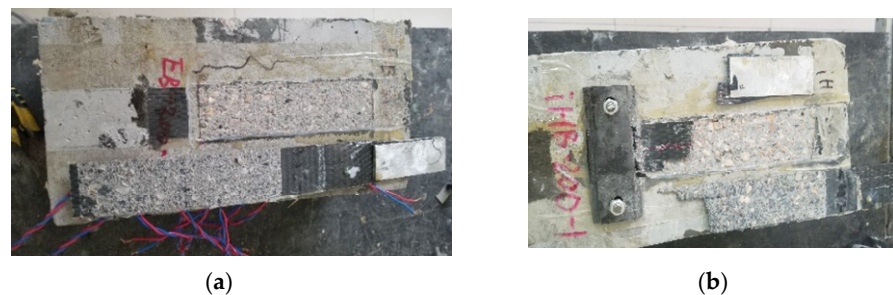
Figure 8. Failure of specimens: (a) EB-200-0; (b) SLHB-200-15.
