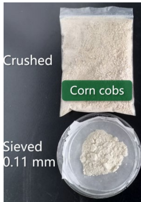
Figure S1 Images of the powder of corn cobs, related to Figure 1 .
