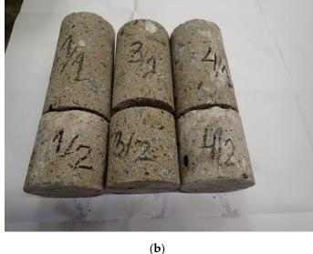
**Figure 3.** Old cylindrical concrete specimens: (a) taken from basement wall using a borehole diamond drill machine; (b) example view on some prepared concrete cores.
