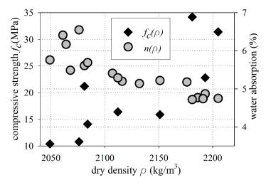
Figure 5. Compressive strength and water absorption vs. dry density.
