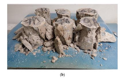
**Figure 7.** Frost resistance tests: (a) view of concrete specimens inside the freezing chamber after tests; (b) view of a form of failure concrete specimens.
