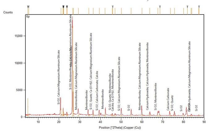
Figure 13. XRD pattern of the old concrete sample.
