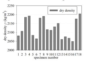
Figure 4. Measurement of the old concrete dry density.
