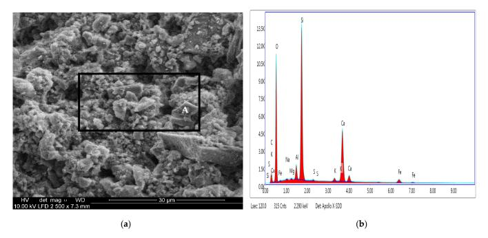
**Figure 12.** SEM/EXD analysis: (a) SEM microscopic images; (b) EDS of the sample on the selected area (A).
