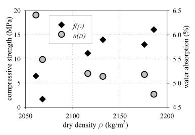
Figure 8. Compressive strength after 50 freezer cycles and water absorption vs. dry density.
