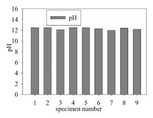
**Figure 10.** The pH value of the old concrete.
