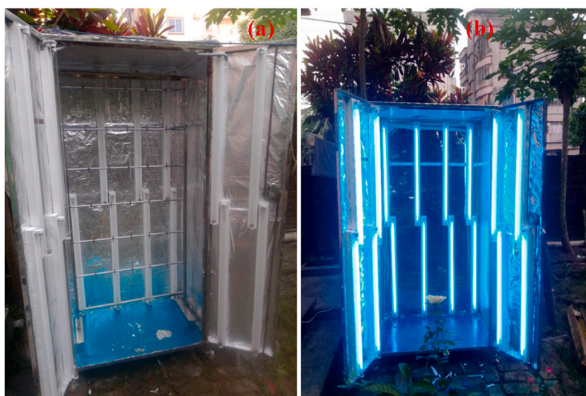
Fig. 1. Final prototype of UVC disinfection chamber. The image left without illumination (a) and right after illumination (b) shows the UV-C chamber.
