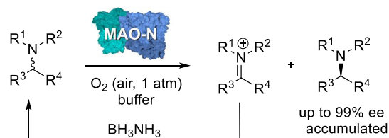
Figure 3. General scheme for dynamic kinetic resolution or deracemization: MAO-N catalyzes the oxidation of primary, secondary, and tertiary amines, followed by chemical nonselective reduction of imines by \text{BH}_3\text{-NH}_3 .
