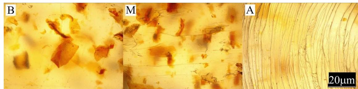
**Figure 8.** The appearance of individual parts of the injection moulding obtained with a 5% content of bran fraction with a grain size of 0.4–0.6 mm at measuring points A, M, B (the position of the points is marked in Figure 1).
