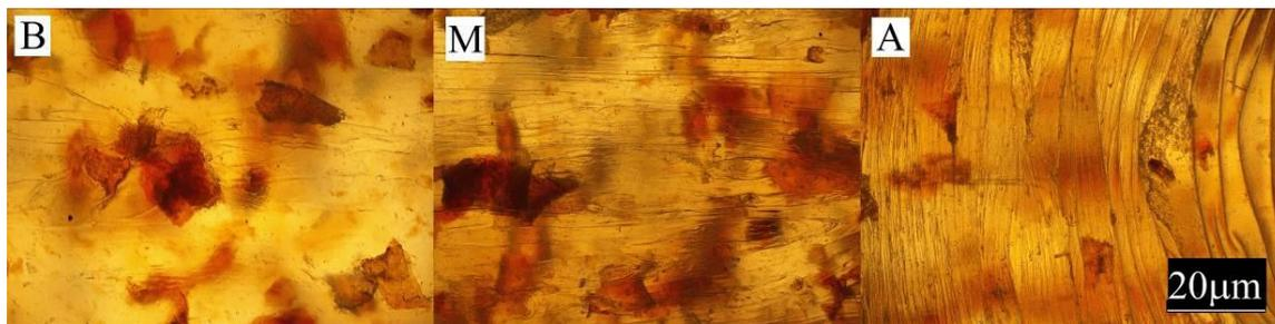
**Figure 9.** The appearance of individual parts of the injection moulding obtained with a 15% content of bran fraction with a grain size of 0.4–0.6 mm at measuring points A, M, B (the position of the points is marked in Figure 1).
