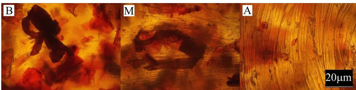
**Figure 11.** The appearance of individual parts of the injection moulding obtained with a 15% content of the bran fraction with a grain size of 0.6–0.8 mm at measuring points A, M, B (the positions of the points are marked in Figure 1).
