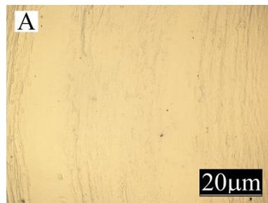
**Figure 12.** Appearance of the unfilled polyethylene moulding at measuring point A (the position of the point is marked in Figure 1).
