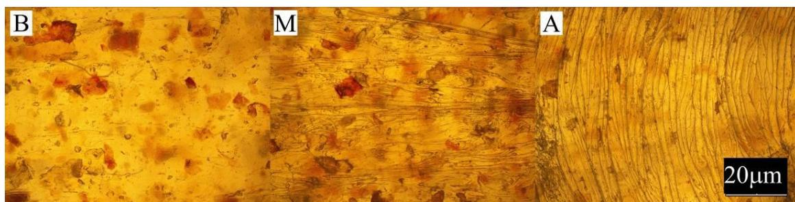
**Figure 7.** Appearance of the individual parts of the injection moulding obtained with a 15% content of bran fraction with grain size < 0.4 mm at measuring points A, M, B (the positions of the points are marked in Figure 1).
