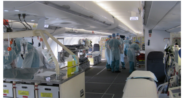
Fig. 1. PHENIX plane medically equipped with the MoRPHEE systems. Photo credits: Mathieu Boutonnet.
