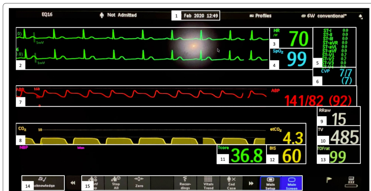
Fig. 1 Conventional monitor configuration investigated with eye-tracking in this study. White numbered boxes indicate the predefined areas of interest. 1: Time; 2: electrocardiogram (ECG); 3: heart rate (HR); 4: oxygen saturation (SpO2); 5: ST-analysis of electrocardiogram (ST-Analysis); 6: central venous pressure (CVP); 7: Arterial blood pressure (ABP); 8: end-tidal carbon dioxide concentration (etCO2); 9: respiratory rate (RR); 10: tidal volume (TV); 11: temperature (Temp); 12: bispectral index (BIS); 13: train of four peripheral nerve stimulation (TOF); 14: Button for alarm acknowledgment; 15: Patient monitor settings (PM)
