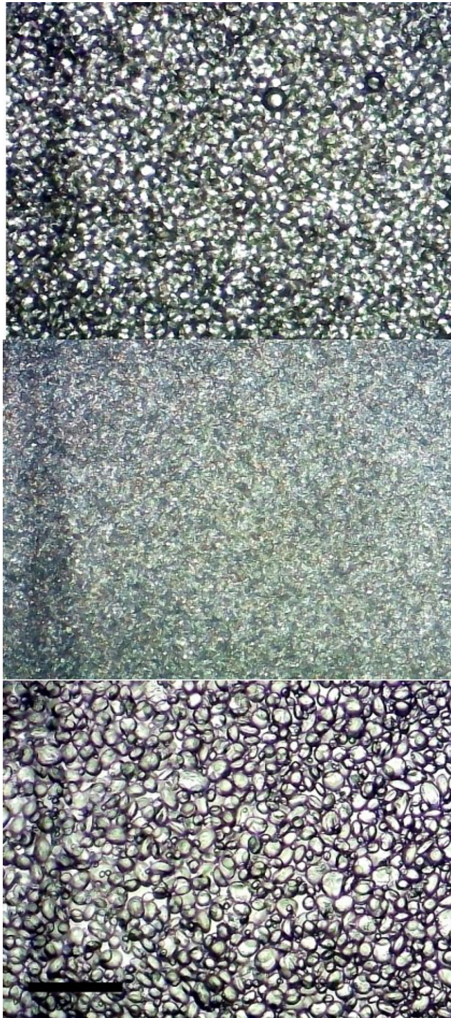
Fig. 7. Microscopy of starch from different sources. Top to bottom – 50% HES in water; 50% starch from rice in water; 50% starch from wheat in water. Scale bar is 100 \mu\text{m} . Images were taken in a static system, where no shear was applied.
