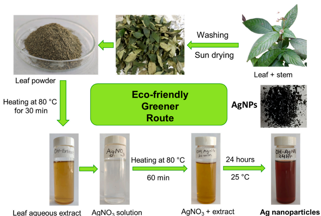
Fig. 2. Schematic representation of the synthesis of AgNPs from the aqueous leaf extracts of three Ophiorrhiza species.
