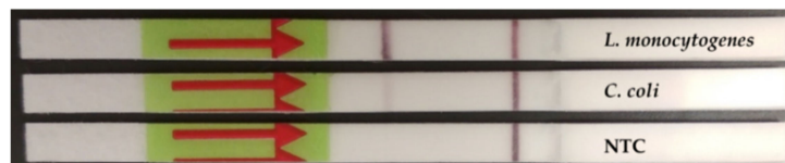
Figure 2. Lateral flow strips showing the difference in the intensity of the test band with a specific ( L. monocytogenes ) and non-specific ( C. coli ) detection obtained with RPA amplification, using PCR primers. NTC: non-template control.
