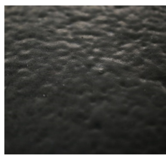
(e) Bumpy and wobbly surface of CB-40 after decompression
