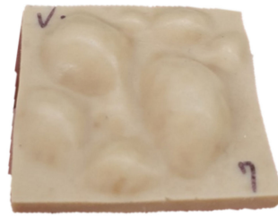
(b) Severe blisters occurring in non-filled NBR
