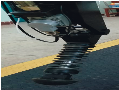
FIGURE 8: Single leg of the hydraulic quadruped robot.
