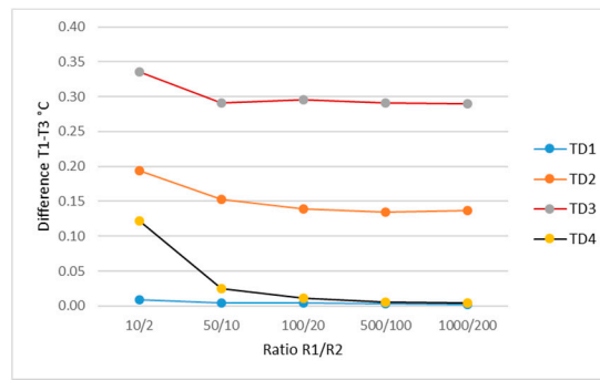
Figure 6. Influence of thermal channels materials’ thermal conductivity on the material temperature at the boundary between the tissue surface and the transducer pad.
