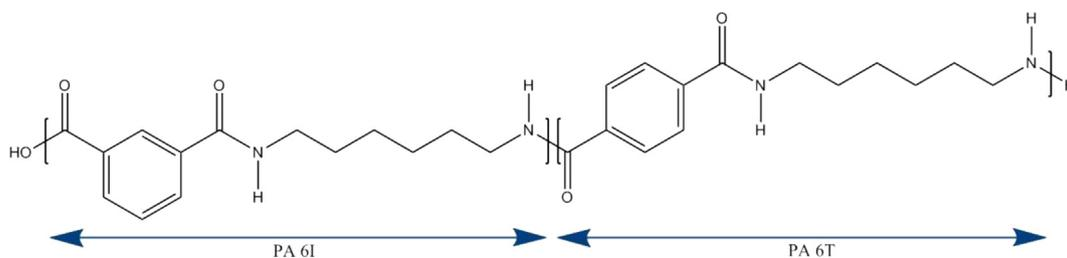
Figure 1. Structure of the copolymer PA6I/6T.
