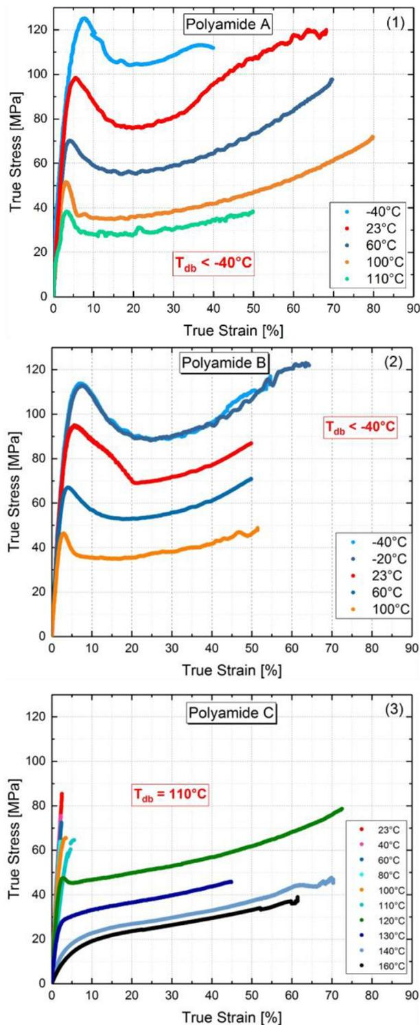
**Figure 7.** Uniaxial tensile true stress-true strain curves determined for Polyamide A (1), Polyamide B (2) and Polyamide C (3) at several temperatures and a strain rate of  $1.10^{-3}$  s<sup>-1</sup>.
