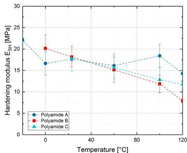
**Figure 10.** Evolution of the hardening modulus  $E_{SH}$  in compression with the temperature for each PPA. The modulus  $E_{SH}$  was determined from the slope of the curves in the strain range 1.25–1.75.
