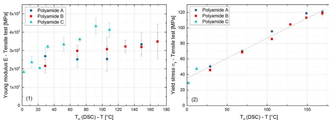
**Figure 8.** Evolution of the Young modulus  $E$  (1) and the yield stress  $\sigma_y$  (2) as a function of  $T_g - T$ . Data are obtained from tensile measurements at a constant strain rate of  $1.10^{-3} \text{ s}^{-1}$ .
