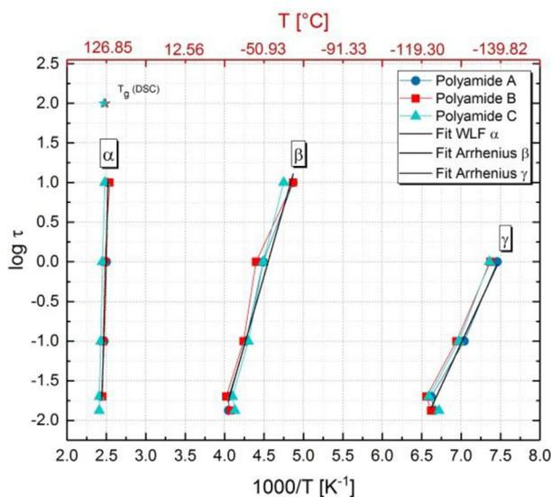
**Figure 5.** Time/temperature dependence of relaxations for the three PPA. From left to right, the different relaxations are shown:  $\alpha$ ,  $\beta$  and  $\gamma$ , as well as the  $T_g$  determined by DSC.
