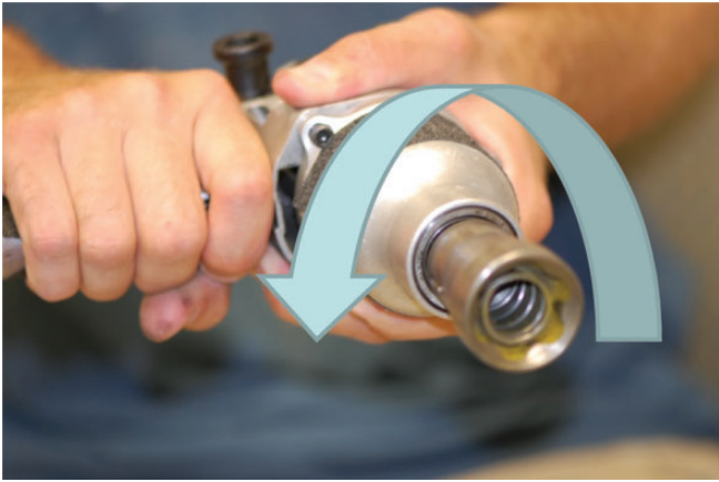
Figure 1. Air-powered impact wrench vector of force exerted on NASCAR changers causing torsional wrist injuries.
