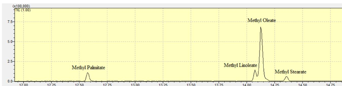
**Figure 1.** GC chromatogram of fatty acid methyl esters of biodiesel synthesized from waste cooking oil and grease (DB-5 ms column).
