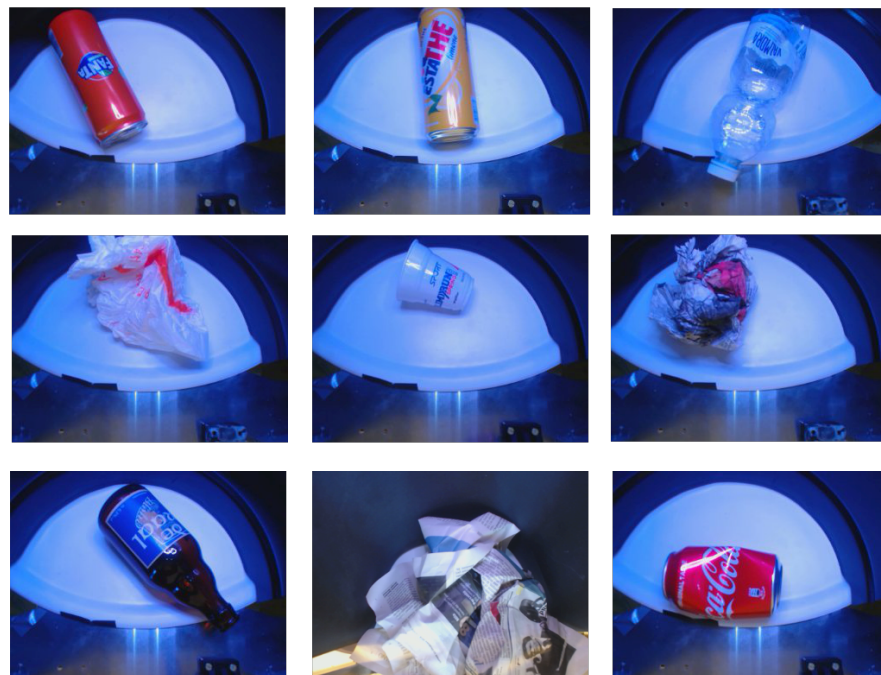
Figure 8. A sample of the pictures used as training dataset. The objects were acquired by the waste sensing module directly on the white shelf of the waste disposal unit.
