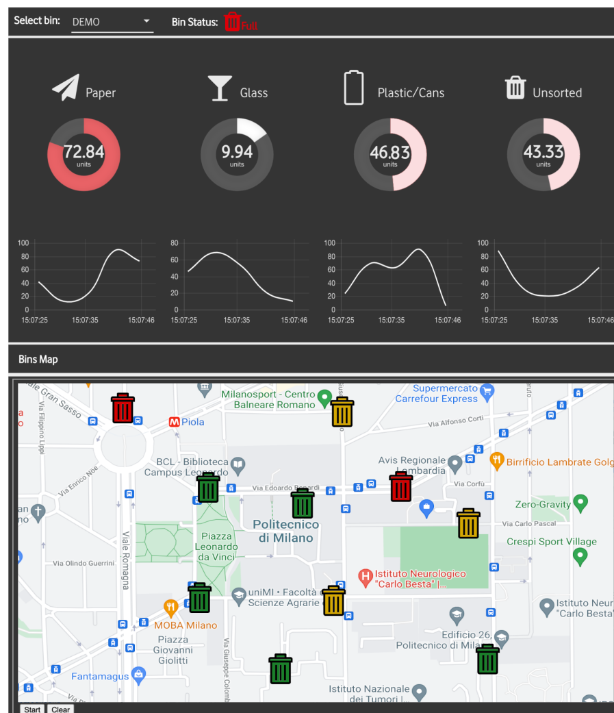
Figure 13. Smart waste bin backend dashboard implemented with Node-RED. The map shows the bins' position as well as a graphical summary of the fill levels. Respectively, red when at least one class is greater than 70%; yellow when at least one class is greater than 40% and green when all the classes are below or equal 40%.
