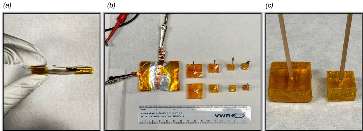
Supplementary Figure 4. Triboelectric tactile sensor and touch stimuli. a) Side view of the tactile sensor, with Kapton on the bottom layer on top of a supporting substrate with spacers separating it from the top aluminum layer sitting below a separate supporting substrate. b) Top view of the tactile sensor with copper extensions from the top and bottom layer and PDMS stamps used for the experiment representing different touch stimuli. c) Closer image of PDMS stamps.
