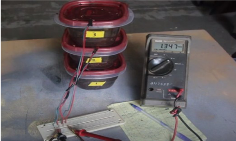
Fig. 1. MFC set up used for the experimental tests. Source: photo credit by the present authors.
