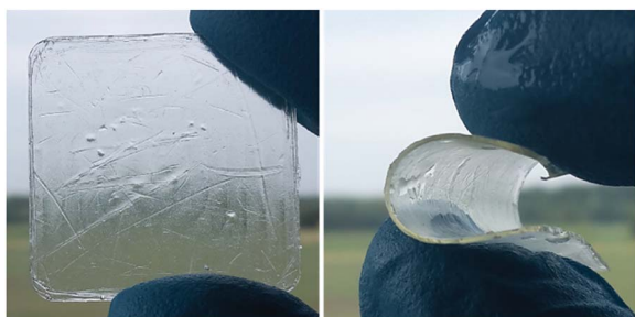
Fig. 5 Pictures for XUrDMA1 before (left) and after (right) immersion in PBS.
