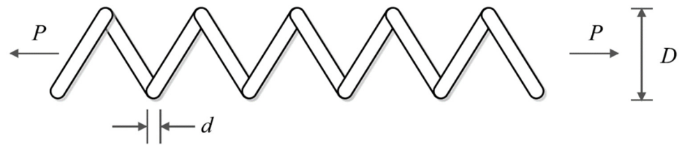
Figure 14. Schematic of the tension/compression spring design.
