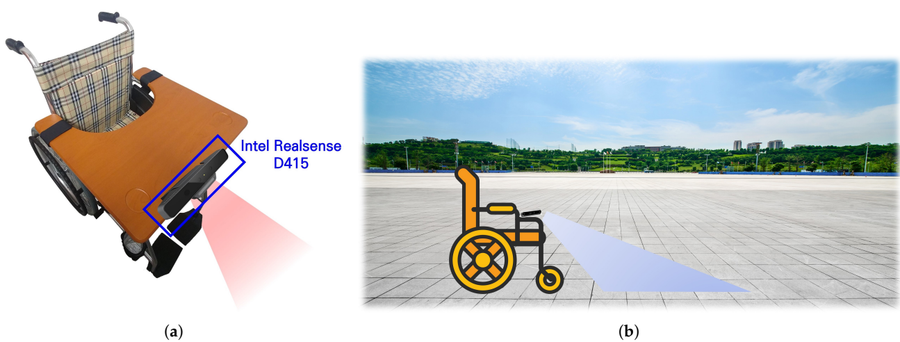
Figure 1. Wheelchair setup. (a) Hardware setup, (b) Recording configuration.
