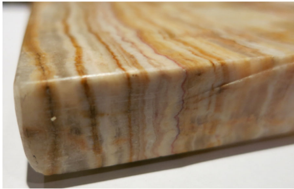
Fig. 1 Two orthogonal faces of planar layers of marble. By inspecting both the top and side, it is possible to infer that the rust-colored forms that appear as lines on each face are the visible expression of 3D planar layers that extend through the object
