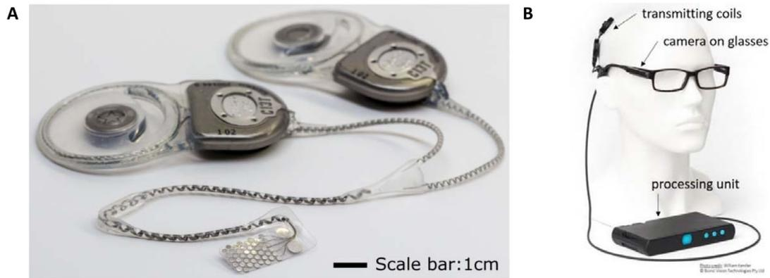
**Figure 1.** (A) The implanted ocular electrode array (left eye variant) shown with two implantable stimulators (image courtesy of D.A.X. Nayagam). (B) External components including a spectacle-mounted CMOS video camera, head-worn magnetically coupled transmission coils, and a body-worn portable video processor (image courtesy of W.G. Kentler).
