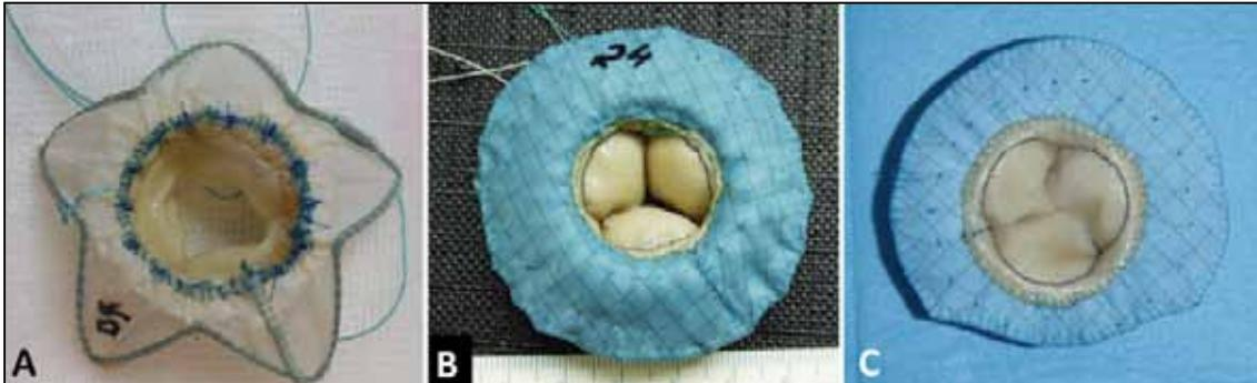
**Figure 2** - Different prototype designs resulting from iterative development of the mitral valved stent. A: valved stent with star shaped atrial element; B: valved stent with crown shaped atrial element attached at  $45^\circ$  to the ventricular element, C: valved stent with a D-shaped atrial element for better alignment in the antero-medial area.
