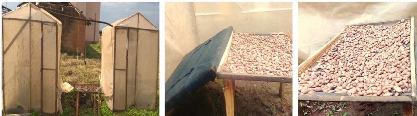
FIGURE 1 Prototype greenhouse dryers (left), internal view of MGHD (modified greenhouse) showing position of the fleece (middle), and CGHD (conventional greenhouse) (right)
