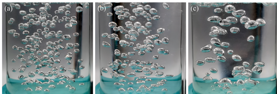
Figure 4. Bubble distribution at 90 L/h with different gas distributors: (a) T-1; (b) T-2; (c) T-3.
