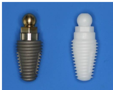
Figure 1. Images of the Ti (left) and ZC one-piece implants (right).
