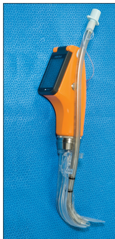
Figure 1: Pentax airway scope; tracheal tube loaded into the integrated tube channel of the P blade
