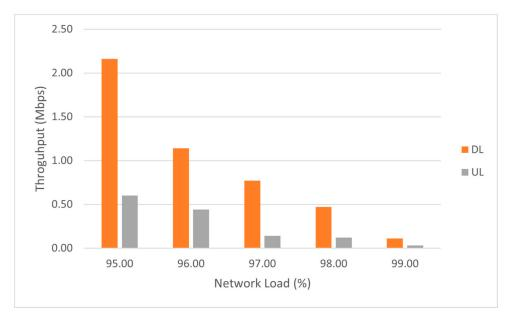
Figure 25. The UE throughput variation in case of high network load on UPF.
