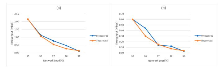
**Figure 26.** Comparison of UE throughput between the measured value and the value predicted by (9) in case of network load higher than 95%. (a) Downlink. (b) Uplink.
