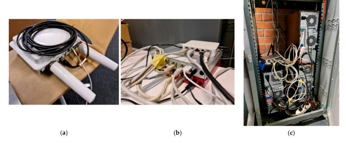
Figure 8. E2E experimental testbed. (a) Nokia FZM eNB. (b) Open vSwitches. (c) OpenStack private cloud.
