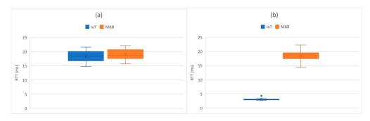
**Figure 20.** Comparison in RTT variation between IoT and MBB traffic: (**a**) when using the same link; (**b**) after the network congestion detection feature is enabled.
