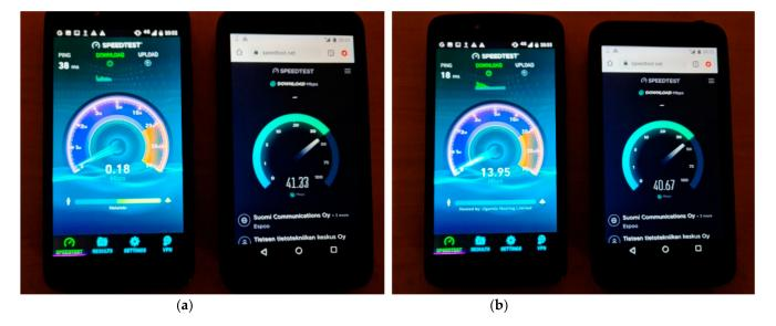
**Figure 23.** The throughput difference for the UEs connected to different UPFs. (**a**) The load of the previous UPF is almost 100% (left image). (**b**) The load of the previous UPF is approximate 70% (right image).
