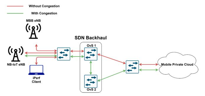
address for the incoming packets is set on the OvS 1 in order to forward the IoT traffic to the OvS 2 and from there to the cloud.
