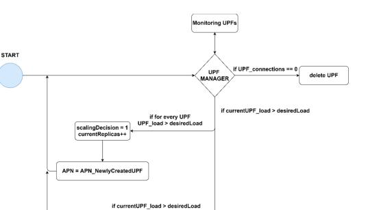
Figure 11. The proposed scaling algorithm for UPF.
