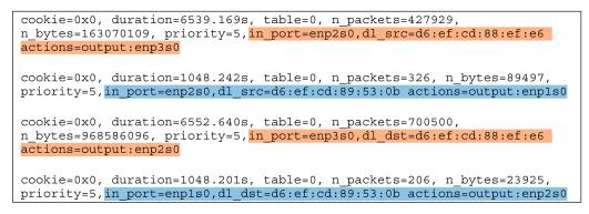
Figure 19. Flow table for OvS 1 after network congestion.
