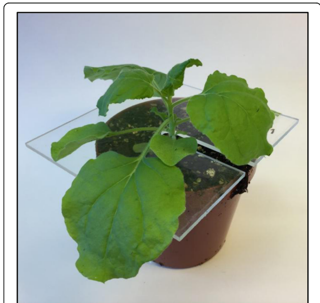
Fig. 4 Acrylic seal used to enclose soil during vacuum infiltration of N. benthamiana . The acrylic sheet (130 × 130 mm) prevented soil from upturned plants from falling into the infiltration medium
