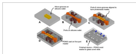
**Figure 1.** Schematic showing fabrication of the microfluidic device. (A)–(C): Photolithography was used to fabricate the master. (D)–(E): Soft lithography was used to inversely replicate the master and produce the devices. Holes indicated by blue arrowheads in E allowed access to microfluidic devices and were drilled into PDMS moulds before sealing the devices to glass cover slides.
