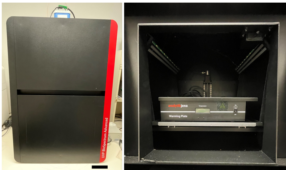
Figure 2. External and internal view of the Analytik Jena UVP Biospectrum Advanced system. Left; External view. Right: Internal view). Scale bar: 10 cm.
