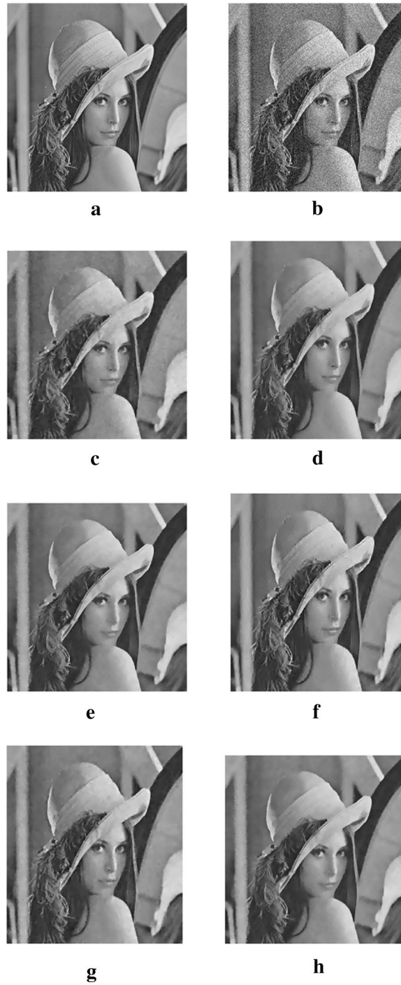
Fig. 4 Results of Lena image by the six models. a Original image, b noisy image, c result by TV model, d result by LLT model, e result by NLM model, f result by BLS-GSM model, g result by hybrid model, h result by our model
