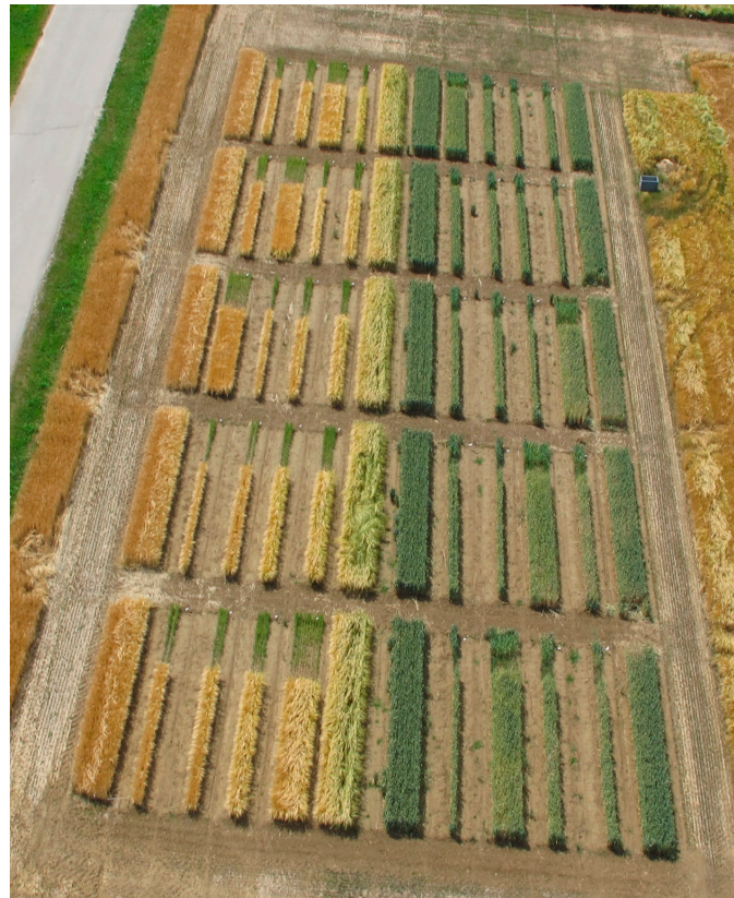
Figure 2. UAV image of the field trial. Different plot designs, including one-, two-, three- and four-row designs, were tested using winter wheat and winter barley as crops.
