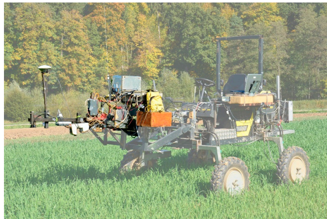
Figure 4. Sensor carrier PhenoTrac IV, customized by the Chair of Plant Nutrition from the Technical University of Munich.
