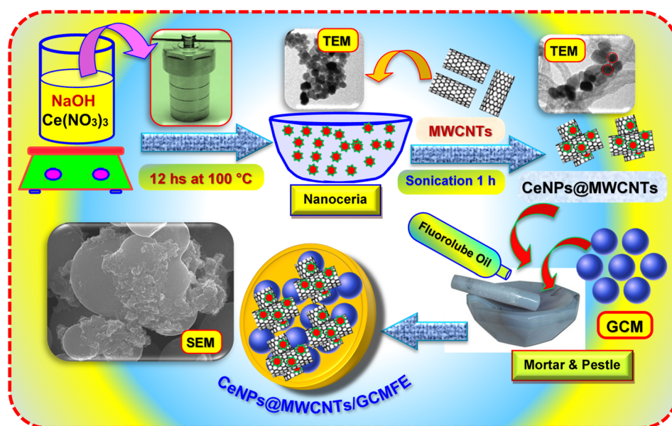
Scheme 1 Schematic diagram of preparation process of CeNPs@MWCNTs modified GCMFE.
