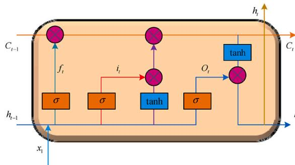
Fig. 3. Unit structure diagram of LSTM.
