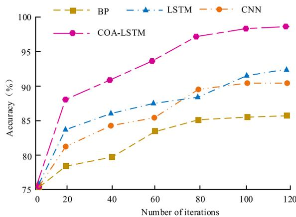
Fig. 6. Comparison outcomes of prediction precision of the four selected methods in the same dataset.
