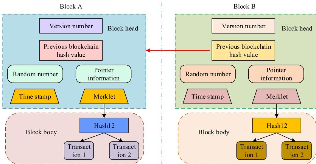
Fig. 1. Fundamental structure of blockchain network.
