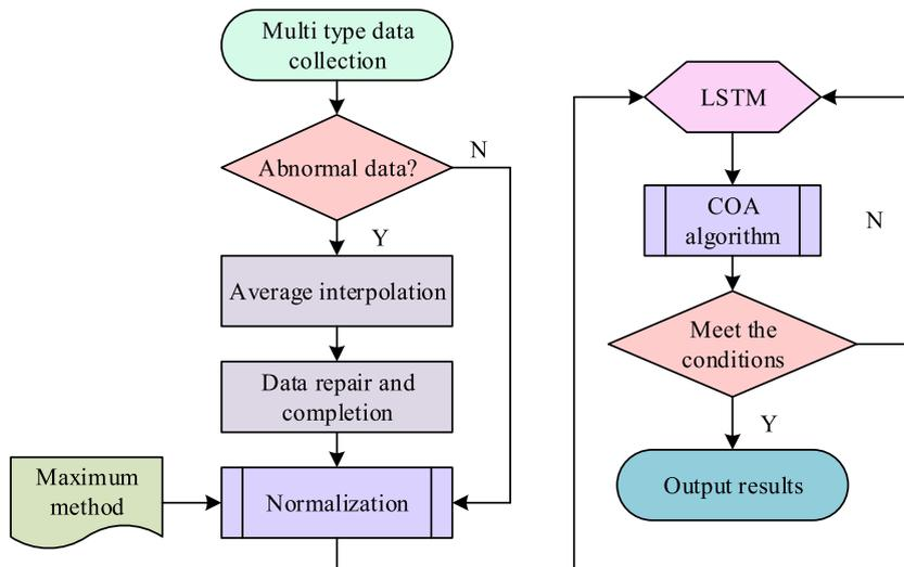
Fig. 4. The upgraded LSTM carbon emission prediction process.
