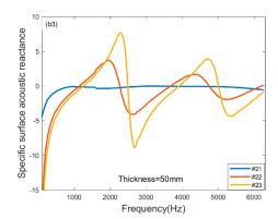
**Figure 4.** Sound absorption measurement of molecular sieve pellets with different pellet sizes. Sound absorption coefficients of 5Å with thickness of (a1) 30 mm; (b1) 50 mm; Specific surface acoustic resistance of 5Å with thickness of (a2) 30 mm; (b2) 50 mm; Specific surface acoustic reactance of 5Å with thickness of (a3) 30 mm; (b3) 50 mm.
