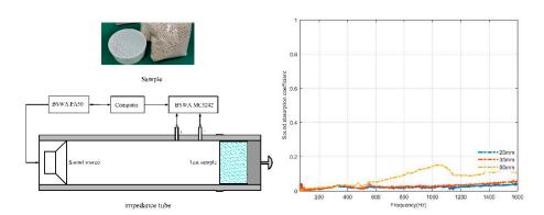
**Figure 1.** Experiment setup. On the left are the sample and the impedance tube, and on the right is the absorption coefficient of the cylindrical box.
