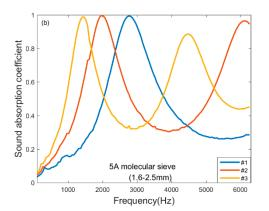
**Figure 3.** Sound absorption measurement of molecular sieve pellets with different thickness: (a) 3Å with pellet size of 3–5 mm; (b) 5Å with pellet size of 1.6–2.5 mm.
