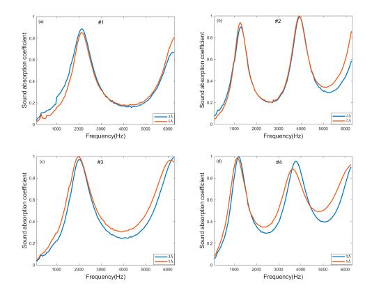
**Figure 2.** Sound absorption measurement of molecular sieve pellets of different pore size. Sound absorption coefficient of 3Å and 5Å with (a) thickness of 30 mm and pellet size of 3–5 mm; (b) thickness of 50 mm and pellet size of 3–5 mm; (c) thickness of 30 mm and pellet size of 1.6–2.5 mm; (d) thickness of 50 mm and pellet size of 1.6–2.5 mm.
