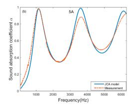
**Figure 5.** Comparison between measurement by impedance tube and estimation through inversion of JCA model. (a) 3Å molecular sieve pellets with thickness of 40 mm; (b) 5Å molecular sieve pellets with thickness of 50 mm.
