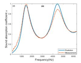
**Figure 6.** Comparison between measurement and prediction for the samples listed in using the inversion parameters estimated in **(a)** new sample #1; **(b)** new sample #2; **(c)** new sample #3; **(d)** new sample #4.
