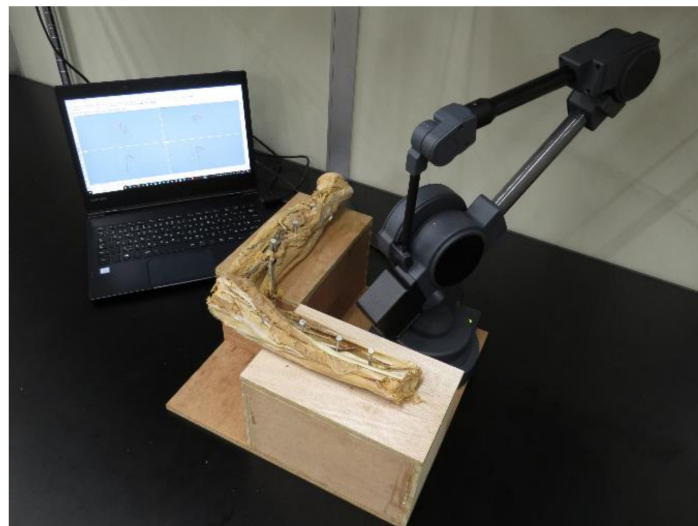
Figure 1. The specimen fixed on the examination table and the MicroScribe system.
