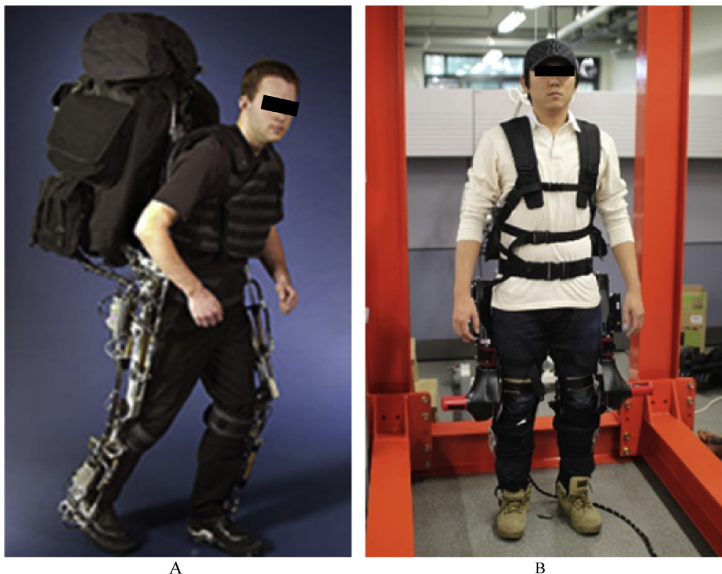
Figure 3 Exoskeletons to augment human strength. (A) The Berkeley Lower Extremity Exoskeleton (BLEEX) (Image credit: Professor Kazerooni of the University of California, Berkeley, CA, USA). (B) The HEXAR-HL35 Exoskeleton (Image credit: Seungnam Yu of the Korea Atomic Energy Research Institute, Daejeon, Korea).
