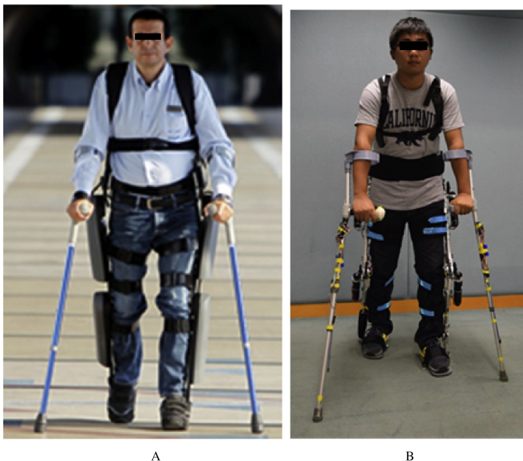
Figure 2 Exoskeletons for locomotion assistance. (A) The ReWalk Wearable System (Image credit: ReWalk Robotics, Inc., Marlborough, MA, USA). (B) The lower extremity exoskeleton developed at the Chinese University of Hong Kong (Hong Kong, China).
