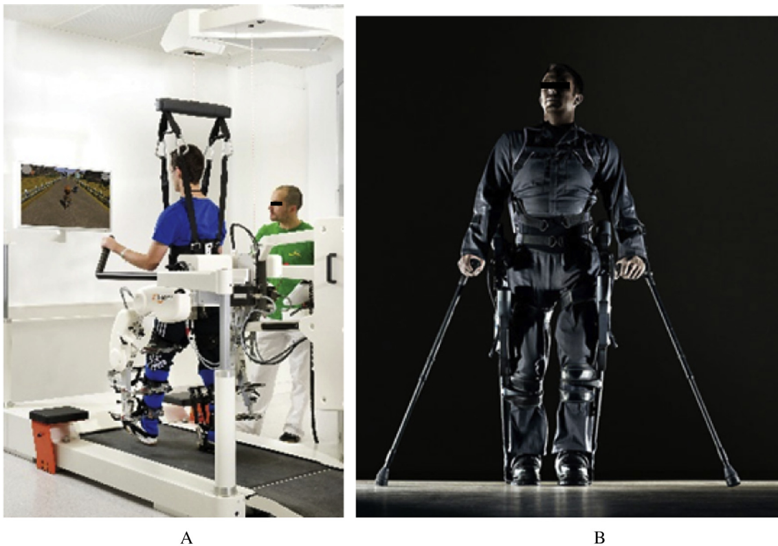
Figure 1 Exoskeletons for gait rehabilitation. (A) The Robotic Orthosis Lokomat (Image credit: Hocoma, Zurich, Switzerland). (B) The Ekso Exoskeleton (Image credit: Ekso Bionics, Richmond, CA, USA).
