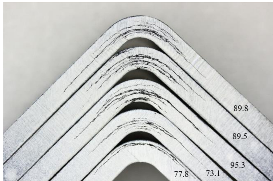
Figure 9. Examples of a typical failure mode for set PPS-CT: the set with the highest coefficient of variation, with the values given in the figure being strengths in MPa.
