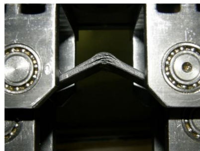
Figure 1. Curved-beam test setup and delamination failure of a polyphenylsulfid (PPS) specimen.
