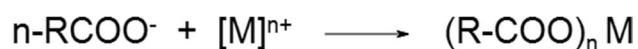
Fig. 4 General representation of the acid–base reaction for the formation of the basic structure of the glass ionomer; M: Ca, Zn, Al; n=2 or 3
