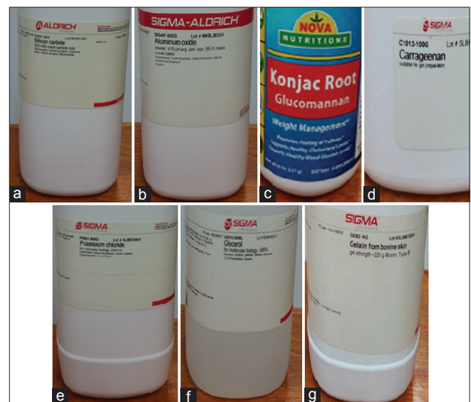
Figure 1: Chemicals items used for tissue-mimicking material flow phantom fabrication: (a) silicon carbide, (b) aluminum oxide, (c) K, (d) C, (e) potassium chloride, (f) glycerol, (g) gelatin
