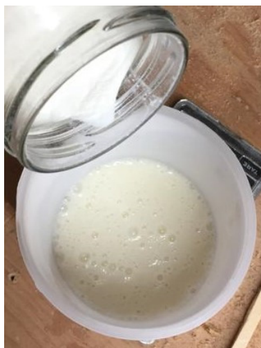
Figure 2. Preparing the adhesive based on casein powder, water, and lime.
