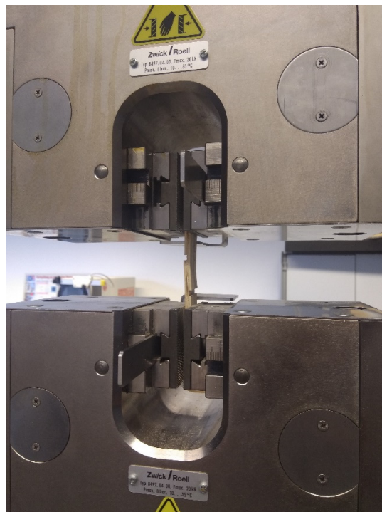
Figure 3. Shear strength test for 3-layer plywood with a Zwick Roell Z250 universal testing machine.
