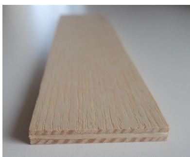
Figure 1. Sample of 3-layer plywood bonded with casein-based adhesive.
