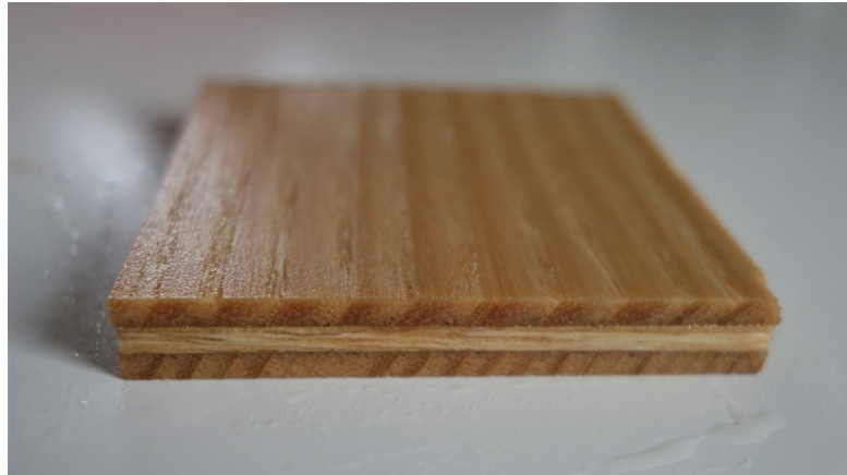
Figure 4. Sample with 3-layer plywood after 24 h water soaking.
