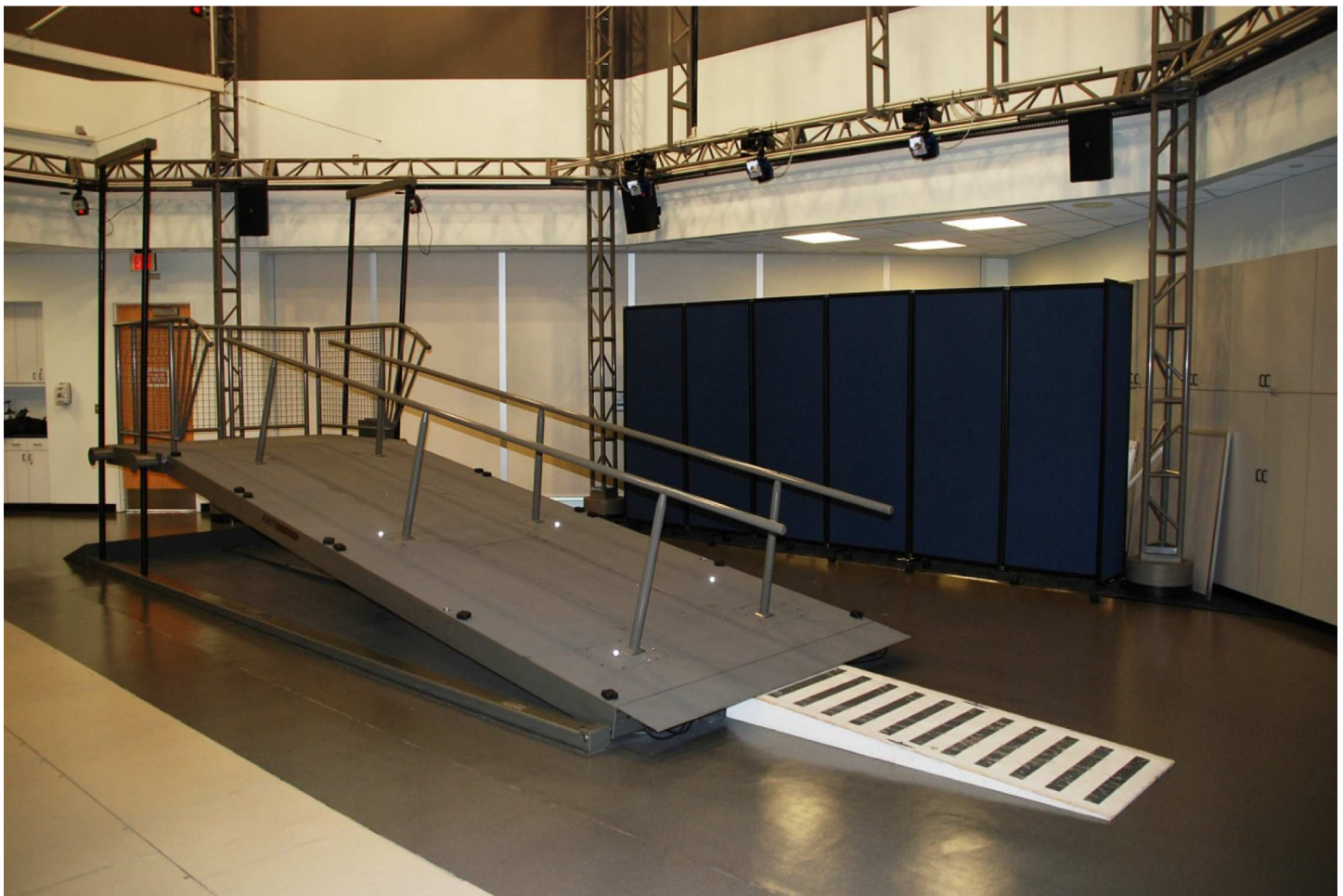
Fig 1. Picture of 5m long instrumented slope that participants walked up.
