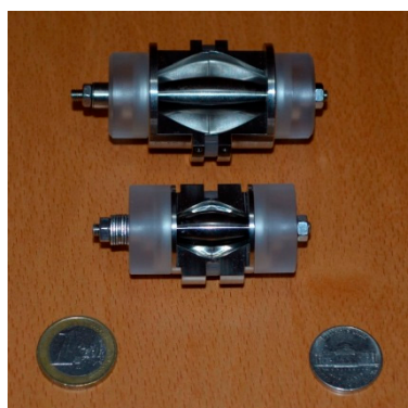
Figure 2. Two Orbitrap analyzers with both a 1-Euro coin and an American nickel as a reference for size [24]. The smaller device is the newer ultra-high resolution Orbitrap analyzer.
