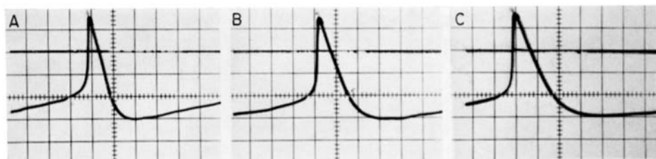
FIGURE 12. Effect of tetrodotoxin on action potential. Records taken from a fiber in solution 4. (A), Control; (B), 40 min after exposure to 10^{-6} g/ml tetrodotoxin; (C), 20 min after exposure to 10^{-5} g/ml tetrodotoxin. Calibration grid: vertical, 20 mV; horizontal, 100 ms.
