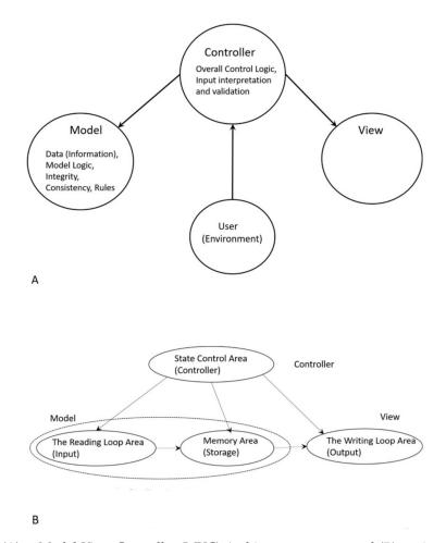
**Figure 12.** (**A**), a Model-View-Controller (MVC) Architecture pattern, and (**B**), an implementation Architecture of von Neumann's Universal Constructor (UC). The solid arrows in the Figure show the flow of control among the components. For example, the solid arrow between the controller and model implies that the controller directs the actions of the model. A dotted arrow indicates a flow of data (information).
